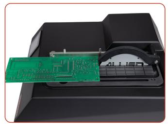
Adjustable table rip fence for measured/guided sectioning
