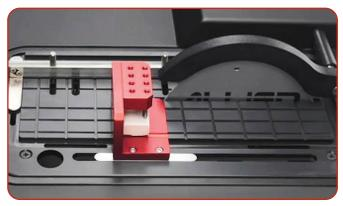
Table slot to guide fixtures for linear cutting
