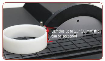
Adjustable blade guard for thick samples
